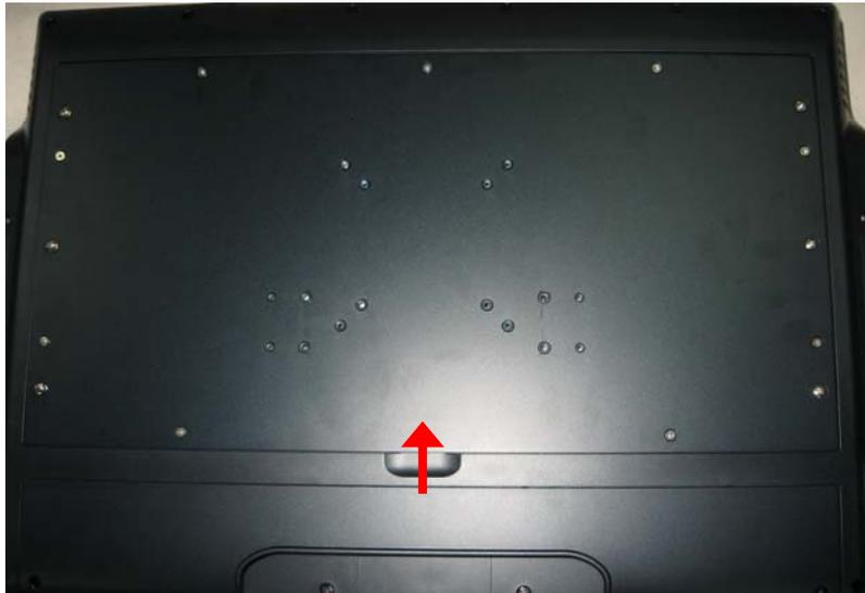
**Step 4** Open the back cover and find mainboard (SBC87830).
