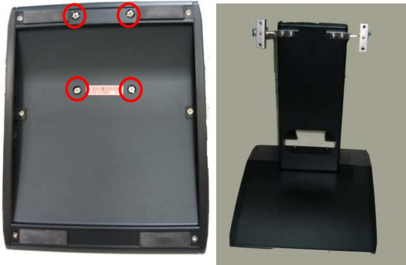
**Step 3** Fix the screws as marked on the back side of chassis (Use Screw B).
