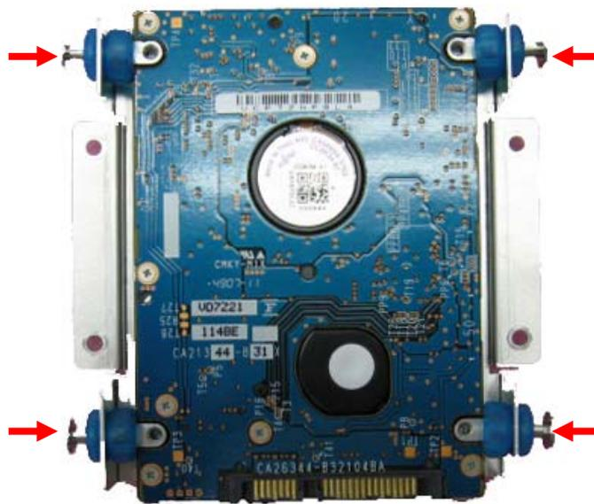
**Step 6** Install the HDD bracket inside the system. Plug the SATA and Power cables in HDD.
