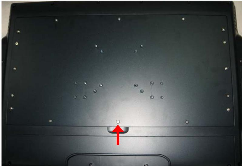
**Step 4** Locate the HDD socket as marked.
